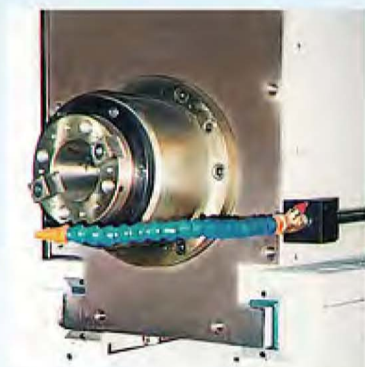
Optional long nose spindle without universal head.
